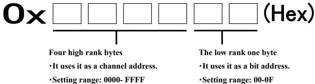
※ To specify only the channel address, the low rank one byte is assumed to be 0x00 and ID is set.
